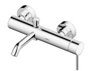
Single lever wall-mounted bath & shower mixer with diverter / brass body, zinc handle /  $\varnothing_{35}\text{mm}$  ceramic cartridge /with aerator / surface treament available with electro-plating, painting, electro-coating, PVD etc.
