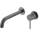
Single lever embeded basin mixer / solid brass body, zinc handle / Ø25mm ceramic cartridge / with aerator / surface treament available with electro-plating, painting, electro-coating, PVD etc.
