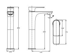
Single lever above counter bidet mixer / brass body, zinc handle / ø35mm ceramic cartridge / with 360° aerator / surface treament available with electro-plating, painting, electro-coating, PVD etc.
