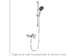
with sliding shower kit / s/s 304 body, zinc handle / ø35mm ceramic cartridge /with aerator / 1.5m shower hose / 3-function handshower / wallmounted sliding bar / surface treament available with electro-plating, painting, electro-coating, PVD etc.
