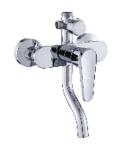
Single lever wall-mounted bath & shower mixer with diverter / brass body, zinc handle / ø35mm ceramic cartridge / s/s spout with aerator / surface treament available with electro-plating, painting, electro-coating, PVD etc.
