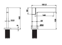
Single lever above counter vessel basin mixer / brass body, zinc handle / cold-open 90° ø26mm ceramic cartridge /with aerator / surface treament available with electro-plating, painting, electro-coating, PVD etc.
