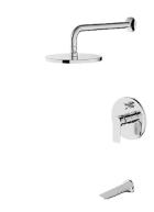
Single lever embeded two-way shower mixer/ brass body, zinc handle / Ø35mm ceramic cartridge / rain shower head and shower arm and spout/ with diverter/ surface treament available with electro-plating, painting, electro-coating, PVD etc.
