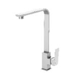
Single lever above counter kitchen sink mixer / brass body, zinc handle / ø26mm ceramic cartridge top sealing /s/s spout with aerator / surface treament available with electro-plating, painting, electro-coating, PVD etc.
