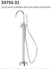
Single lever above counter vessel basin mixer / s/s 304 body, zinc handle / Ø25mm ceramic cartridge /with aerator / surface treament available with electro-plating, painting, electrocoating, PVD etc.
