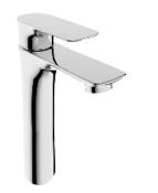
Single lever above counter vessel basin mixer / brass body, zinc handle / Ø35mm ceramic cartridge /with aerator / surface treament available with electro-plating, painting, electrocoating, PVD etc.
