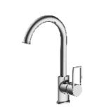
Single lever above counter kitchen sink mixer / brass body, zinc handle / ø35mm ceramic cartridge /s/s spout with aerator / surface treament available with electro-plating, painting, electro-coating, PVD etc.
