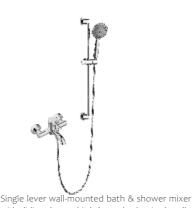
with sliding shower kit / s/s 304 body, zinc handle / ø35mm ceramic cartridge /with aerator / 1.5m shower hose / 3-function handshower / wallmounted sliding bar / surface treament available with electro-plating, painting, electro-coating, PVD etc.
