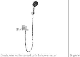
Single lever wall-mounted bath & shower mixer with sliding shower kit /brass body, zinc handle / ø35mm ceramic cartridge /with aerator / 1.5m shower hose / 3-function handshower / wallmounted sliding bar / surface treament available with electro-plating, painting, electro-coating, PVD etc.
