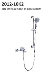
Single lever wall-mounted bath & shower mixer with sliding shower kit / brass body, zinc handle / ø35mm ceramic cartridge /with aerator / 1.5m shower hose / 3-function handshower / wallmounted sliding bar / surface treament available with electro-plating, painting, electro-coating, PVD etc.
