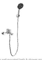
Single lever wall-mounted bath & shower mixer with handshower kit /brass body, zinc handle / ø35mm ceramic cartridge /with aerator / 1.5m shower hose / 3-function handshower / wallmounted shower holder / surface treament available with electro-plating, painting, electrocoating, PVD etc.
