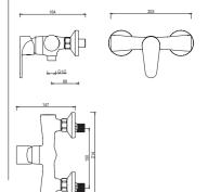
Single lever wall-mounted bath & shower mixer with sliding shower kit /brass body, zinc handle / ø35mm ceramic cartridge /with aerator / 1.5m shower hose / 3-function handshower / wallmounted sliding bar / surface treament available
