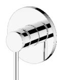
Single lever embeded shower mixer/ brass body, zinc handle / Ø35mm ceramic cartridge/ surface treament available with electro-plating, painting, electro-coating, PVD etc.
